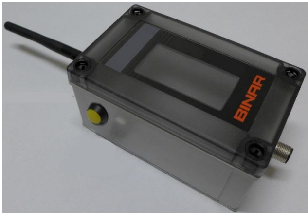
Base unit with antenna, pair button and I/O-connector
